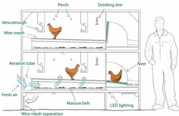
With the two-tiered Veranda Aviary you have full control over your layers. Each tier offers feed, water and nest space, providing easy access for all hens to these essentials. Exterior ramps facilitate access to both levels and the scratching area. The Veranda Aviary:
